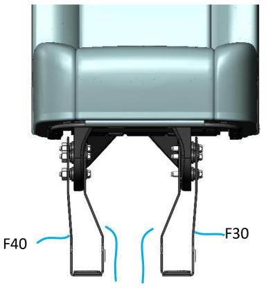
The legs should be attached in such a way that the leg protrude towards inside
