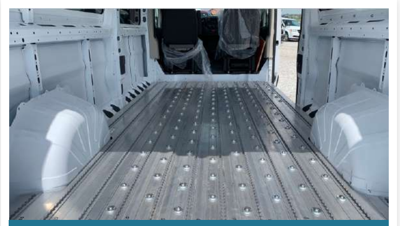
The ball rollers allow moving boxes in any direction in the vehicle.
