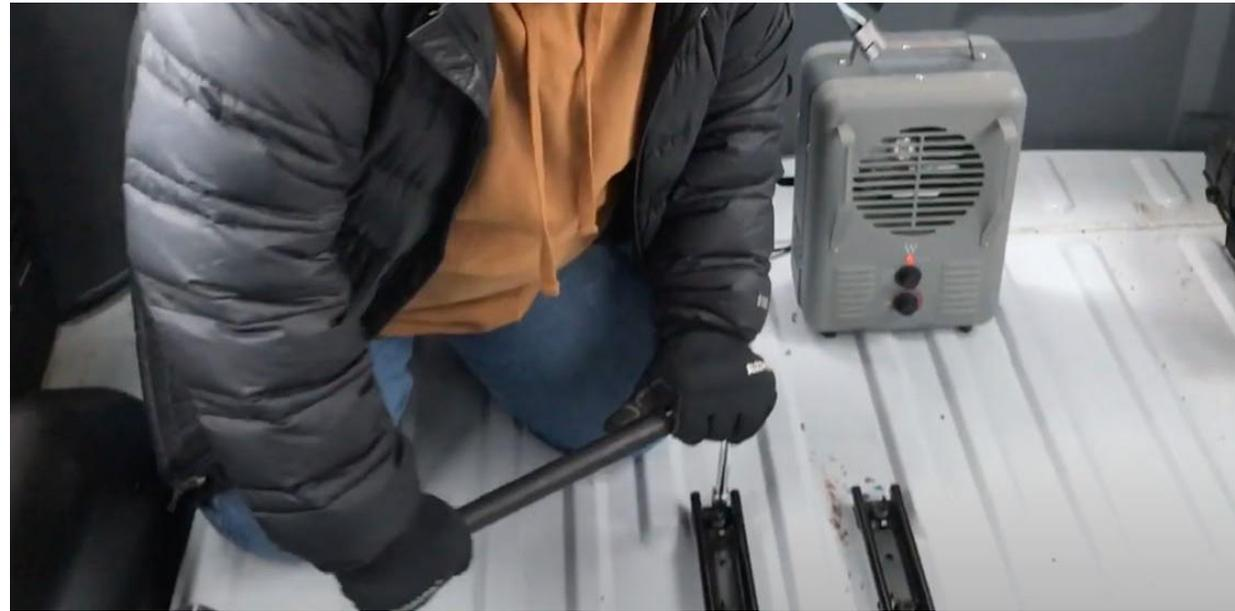
REMOVE THE SCUFF COVER , REMOVE THE FLOOR AND UNBOLT THE OEM SEAT TRACKS
