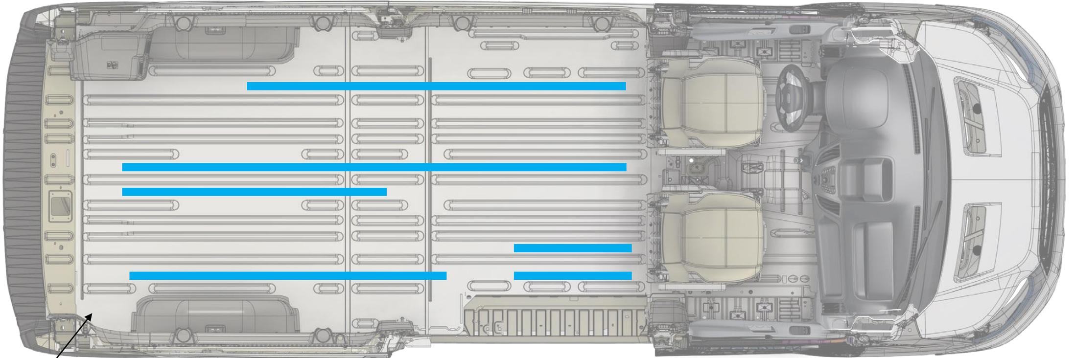
Cover OEM Floor Holes With Silver Duct Tapes
